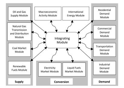
Figure C1: Basic NEMS structure and Information Flow
